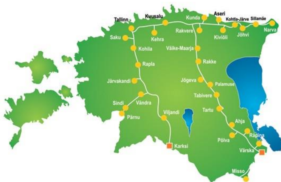
Figure 3.52 Map of high-pressure gas distribution pipelines in Estonia
