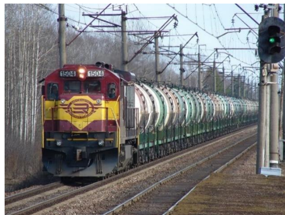
(Photo on the left: Estonian Railways' GE C36-7 diesel-electric locomotive #1504; source: www.bahnbilder.de )
